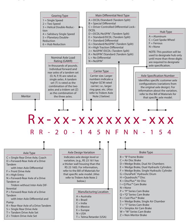
**NOTE 1:** If a complete axle designation is not required, use the first seven positions of the model designation to identify the basic axle model.
